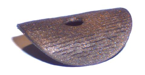
This fuel pump rubber flapper valve was retrieved from a typical mid- to late-1990s model outboard marine engine. The fuel pump experienced total failure, attributed to the valves and other materials hardening as a result of ethanol in the fuel.
