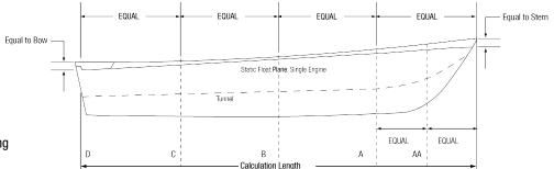
NOTE: Aft end of static float plane determined by lowest point of major leakage; i.e., transom access opening or motor well bulkhead.
