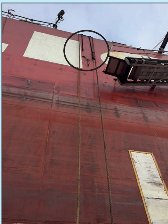
Figure 2: Ladder rigged position, showing broken section
