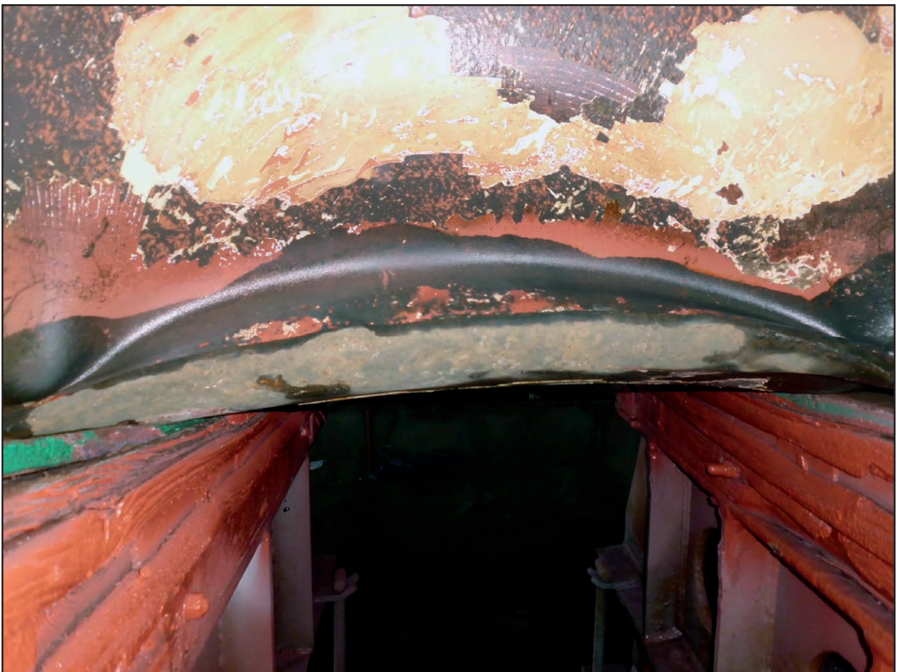
Figure: Hull indentation
