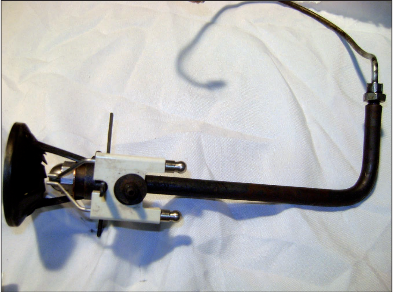
Figure 2: The leaking internal fuel supply pipe to the burner nozzle
