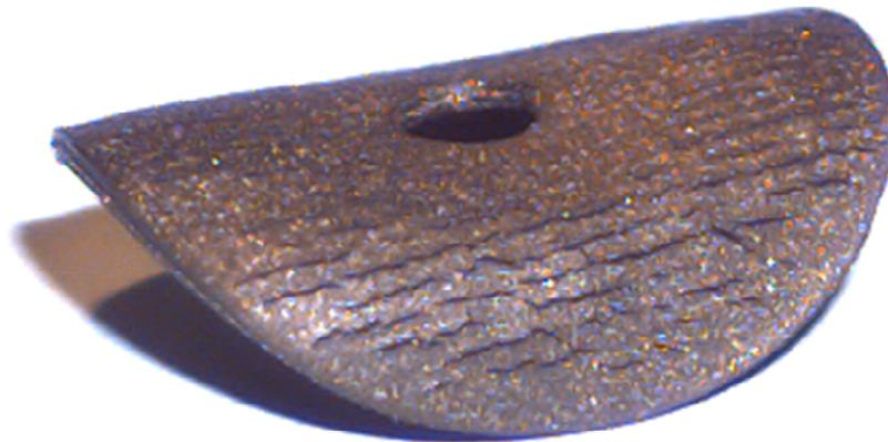
This fuel pump rubber flapper valve was retrieved from a typical mid- to late-1990s model outboard marine engine. The fuel pump experienced total failure, attributed to the valves and other materials hardening as a result of ethanol in the fuel.
