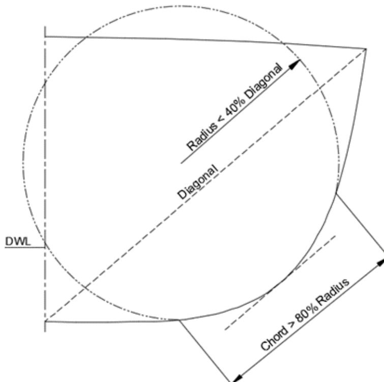
**Figure 3: Natural stiffener criterion for curved panel.**
