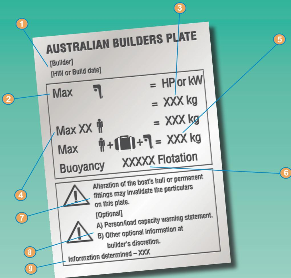
This is a sample ABP plate for a boat less than 6 metres, designed to be powered by an outboard engine, using text and symbols as of 1 November 2005. For further details, please refer to the NMSC web site [www.nmsc.gov.au](http://www.nmsc.gov.au)
