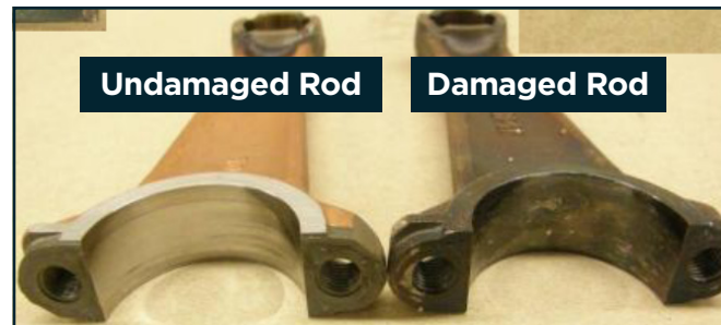
Recovered Pieces from Failed Rod Bearing
