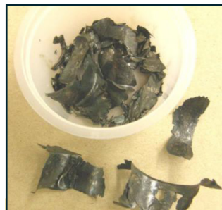
Recovered Pieces from Failed Rod Bearing
