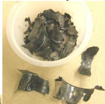
Recovered Pieces from Failed Rod Bearing
