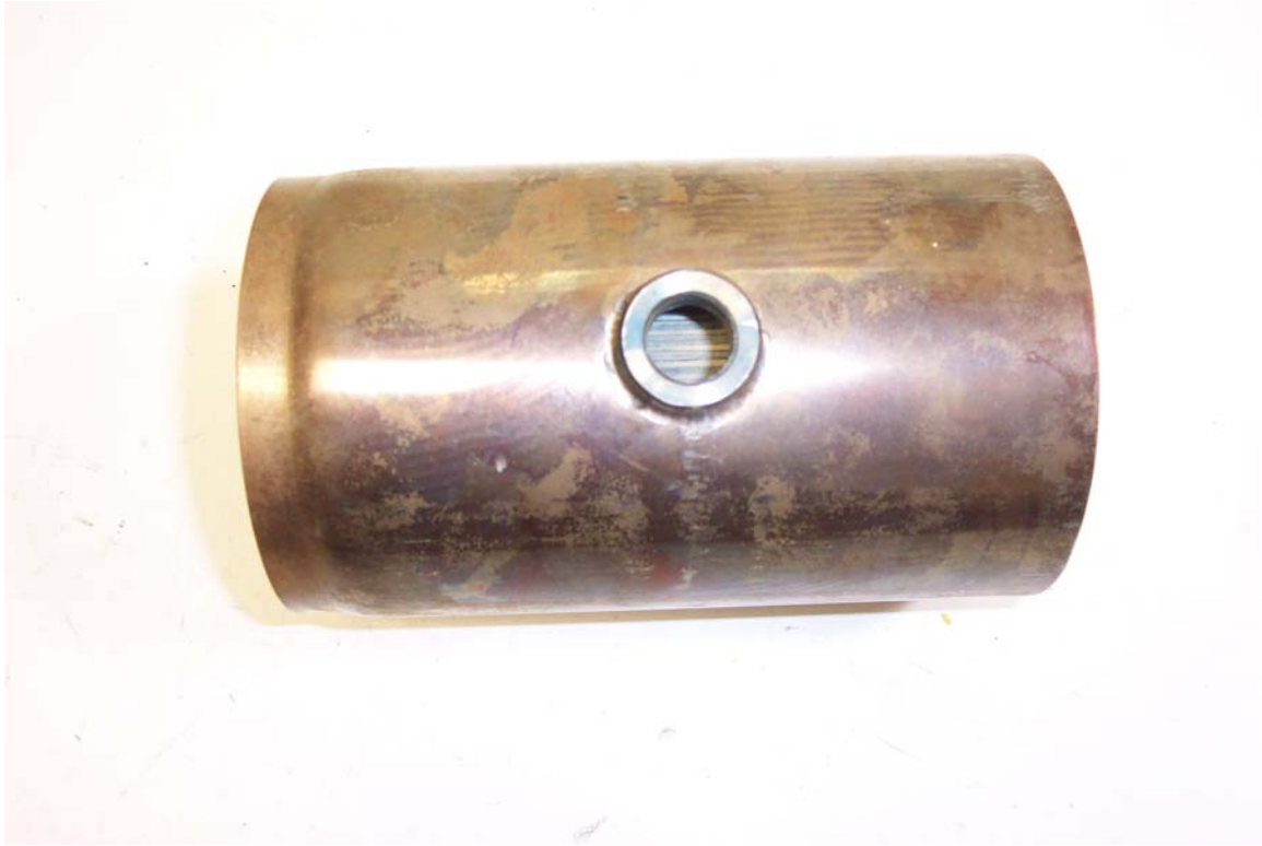
FIGURE 1. METALIC CATALYST WITH HEGO MONITOR BUNG
