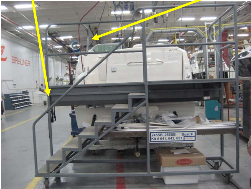
Platform secured to back of boat
